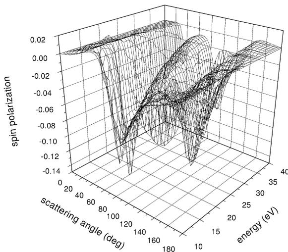
Fig. 4. Three-dimensional plot of the spin polarization cross section for elastic electron scattering from zinc.
