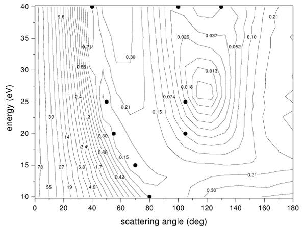
Fig. 2. Contour plot of the present differential cross section for elastic electron scattering from zinc. • indicate positions of experimental minima by Predojević et al. [1].
