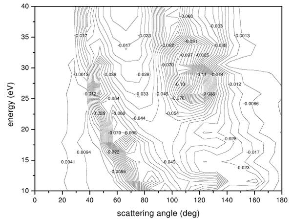
Fig. 5. Contour plot of the spin polarization cross section for elastic electron scattering from zinc.
