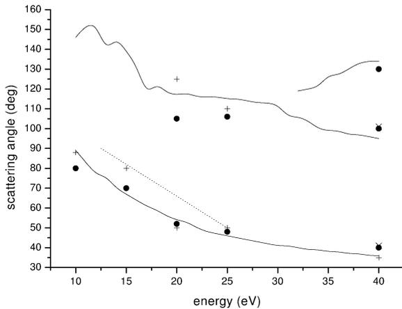
Fig. 3. Positions of differential cross section minima in elastic electron scattering from zinc. Theory: (—) present Letter; (---) McGarrah et al. [5]. Experiment: (●) Predojević et al. [1]; (×) Williams and Bozinis [2]; (+) Childs and Massey [4].
