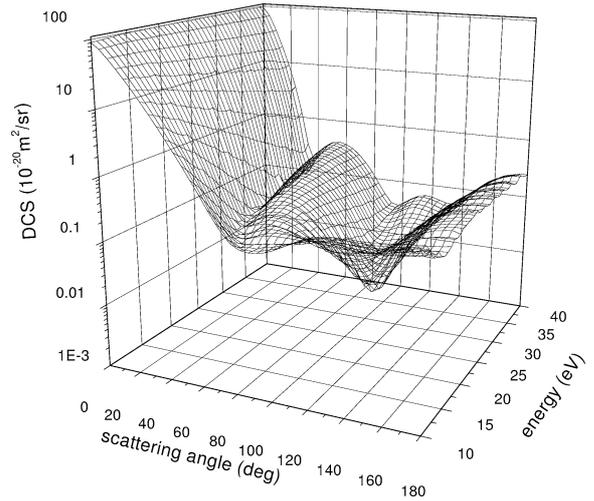
Fig. 1. Three-dimensional plot of the differential cross section for elastic electron scattering from zinc.
